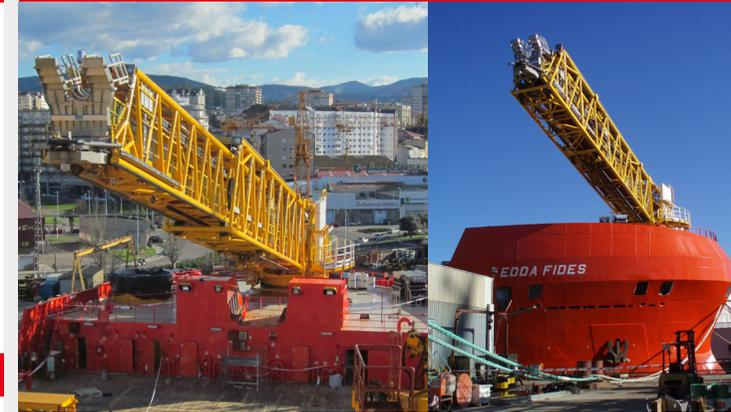
Shell Qatar operates a heave compensated Offshore Access System (OAS) onboard of one of the vessels to serve platforms in the Red Sea. The heave compensated system which maintains the end of the walkway at a constant height is automatically enabled into approach mode when the walkway is slewed outboard from its cradle. In Australia, the OAS allowed uninterrupted access between Marlin B & Edda Fides Flotel during the 8 months KTT Campaign.
