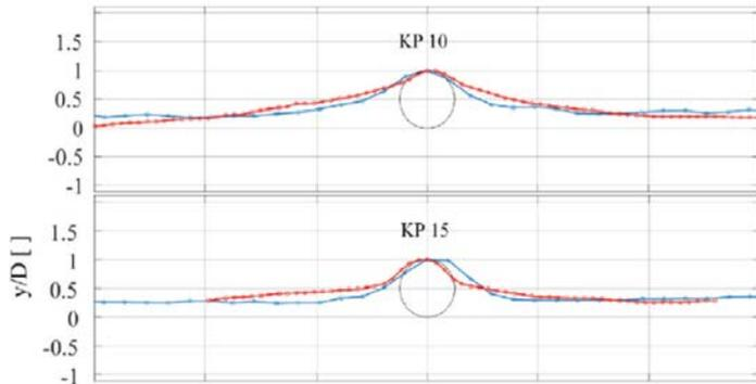
**Top:** pipeline laid with embedment  $\sim 0.1D$ ; after some time, alternating  $0.8D$  local embedment with free-spanning sections (30 – 40 m in length).
