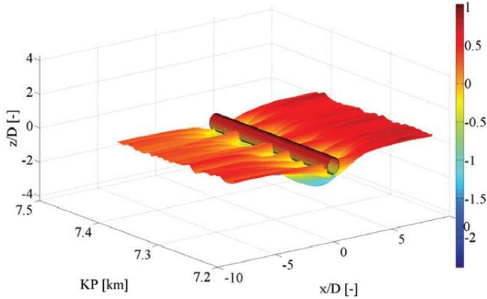
Self-burial or de-burial due to sedimentation and scour affects pipeline on-bottom stability, changes the thermal boundary conditions, affects seabed resistance for buckling design, and can create free-spans.
